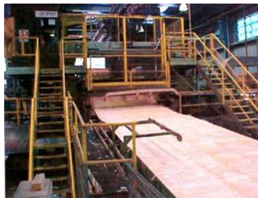
Veneer ribbon exiting lathe after peeling
