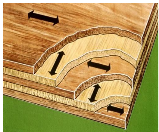
Cross-lamination in plywood as a result of alternating the veneer grain direction of adjacent veneers
