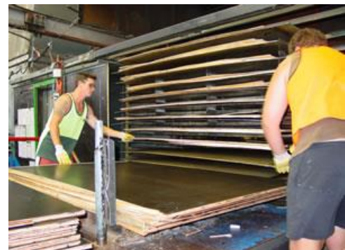
Plywood panels exiting 15 daylight (15 layers of platens) hot press
