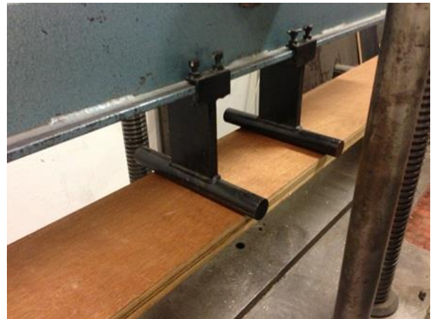
AS 1577: 2013 – Strength Test – Two Line Loads Equidistant about the plank Mid Span
