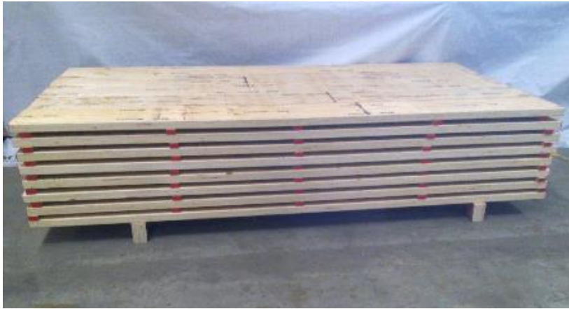
Example of Stacking and Storage conditions for Wet Planks.
