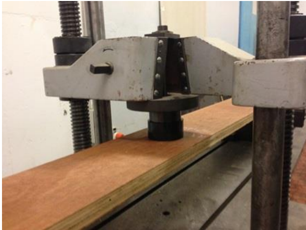
AS 1577: 1993 – Strength Test – Single Point Mid Span
